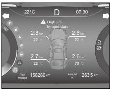
Figure - tire pressure display interface of combination instrument
