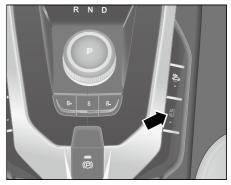
Figure – Automatic parking switch position
