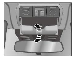
Figure -vehicle top glasses case
