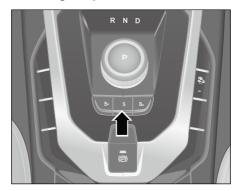
Figure -Partial view of the center console: forward gear sport mode "S"
