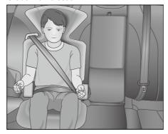
Figure-Grade 2 child seat facing the driving direction
