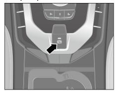
Figure - Electronic Parking Brake Switch Location Manually apply electronic parking:
