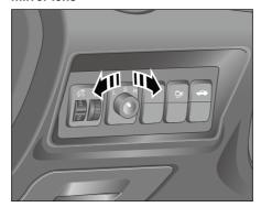
Figure- Exterior Mirror Lens Adjustment Knob
