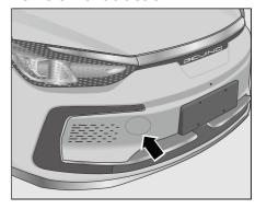
Figure-Vehicle Front Traction Ring Installation Position
