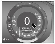
Figure- Trip computer display screen: driving mileage
