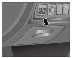
Figure-fuse box in the dashboard
