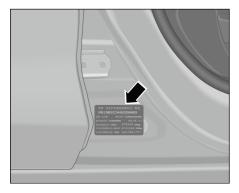
Figure-Location of vehicle nameplate
