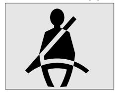
Figure-Driver's seat belt unbelt warning light
