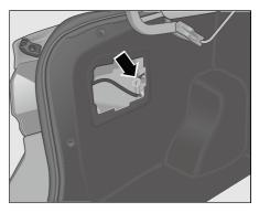
Figure-Emergency Unlock Cable
