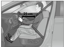
Figure- Distance between driver and steering wheel
