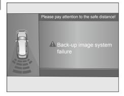
Figure- Non-AVM model backup image failure display
