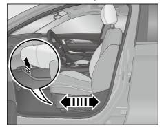
Fgiure-Manually adjust the driver's seat forward and backward
