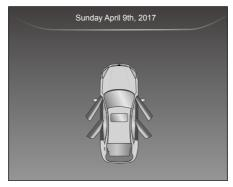
Figure-Reminder that four doors and two covers are not closed
