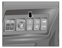
Figure - ESP OFF Button position
