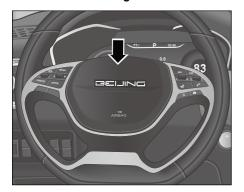
Figure-The driver frontal airbag is installed in the steering wheel.
