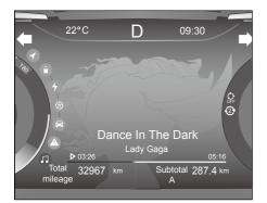
Other information from left to right are driving mileage, engine working time display, transmission oil temperature display (if any) and vehicle voltage display.
