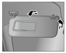
Figure- Driver's Sunvisor: Open and Flip Lower the sunvisor to position to block the light from the front. Put down the sun visor, take out the right side of the sun visor from the clip, and then rotate it to the side to block the light from the side.
