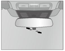
Figure- Adjust the position of manual anti-glare in-vehicle rearview mirror
