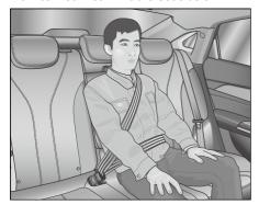
Figure- Correct wearing position of rear seat belt When taking the rear-row middle seat belt, sit straight on the seat and make the back fit the seat back as much as possible. Pull the seat belt out of the retractor, insert the seat belt bolt into the buckle, and belt the seat belt. The bolt clicks when locked in the retractor.
