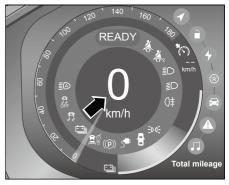
Figure- Trip computer display screen: Digital speed
