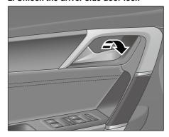
Figure-pull the driver side door handle to open the door
