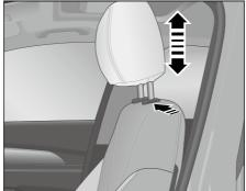
Figure - front seat head restraint adjustment
