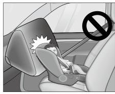
Figure-The inflated airbag slammed into the child seat when the vehicle had an accident
