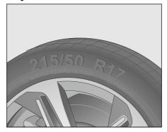
Figure-Tire related information on tire sidewall Check the tire and tire information labels on vour vehicle to find out the tire model and size you need.
