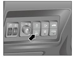
Figure-Hill Descent Control System Switch Button
