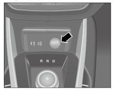
Figure-12V power outlet at dashboard
