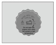
Figure - inside the front engine room: coolant expansion tank cover
