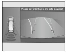
Figure- Non-AVM model parking radar display
