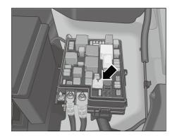
Figure-Fuse puller in front engine room electrical box
