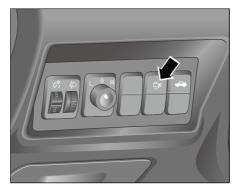
Figure-Hard switch position of panoramic image The left dashboard is equipped with a panoramic image system switch. Press the ON button to turn on the panoramic imaging system. When the system starts, press the ON button again to turn off the panoramic image system.
