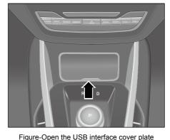
There are two USB interfaces in the front row. Press to open the USB interface cover to see the USB interface.
