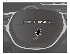
Figure - Multi-function steering wheel right button Press the horn on the steering wheel to mark the area near the horn, the horn will sound, and it will stop when you release it.
