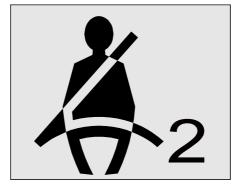
Figure-Front passenger's seat belt unbelt warning light
