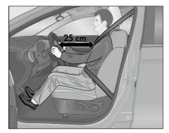
Figure - Correct position between driver and steering wheel
