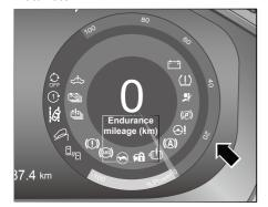
Figure- Trip computer display screen: Wattmeter The virtual pointer dial on the right side of the combination instrument is a wattmeter with an indication range of - 100% ~ 100%. The wattmeter is used to indicate the in-
