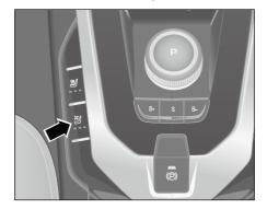
Figure-Seat ventilation button location
