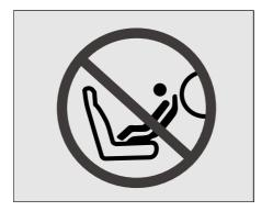
Figure-Warning mark for installation of child seat Do not place the rearward facing child protective device on the front seat, otherwise the back of device will be subject to the great impact energy from the deployment of the airbag, resulting in serious injury or even death.
