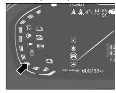
Figure- Power battery electricity meter
