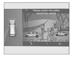
Figure-Low Speed Moving Object Identification Interface
