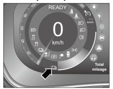
Figure- Trip computer display screen: power battery electricity meter
