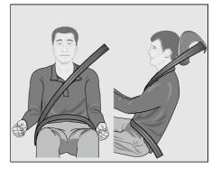
Figure- Correct adjustment position of safety belt
