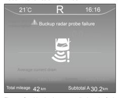
Figure - Combination instrument displays the fault reminder of the parking sensor
